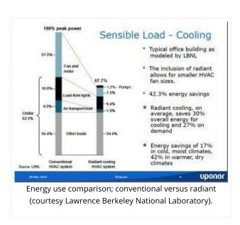
One of the best advantages that radiant cooling systems offer is the potential to lower energy consumption compared to conventional cooling systems. Research conducted by the Lawrence Berkeley National Laboratory in California, has shown significant energy savings potential for radiant cooling, with the amount depending on the climatic area. Their research has shown on average across the USA, savings
