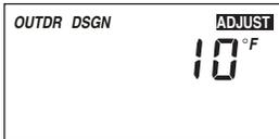
Press and release the **Item** button to advance to the OUTDR DSGN adjustment. Use the ▲ or ▼ button to set the outdoor design temperature. The OUTDR DSGN setting is set to the typical coldest temperature of the year.
