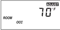
The ROOM OCC adjustment is the first item displayed. Use the ▲ or ▼ button to set the ROOM temperature. The ROOM OCC setting is set to the desired room air temperature during the occupied (Day) mode.
