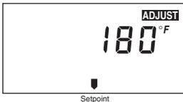
Press and release the **Item** button to advance to the *Setpoint* adjustment. Use the ▲ or ▼ button to set the desired temperature. The *Setpoint* setting is set to the desired setpoint supply temperature.
