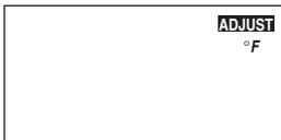
Press and release the **Item** button to advance to the units adjustment. Use the ▲ or ▼ button to set the scale to °F or °C.
