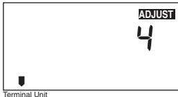
Press and release the **Item** button to advance to the *Terminal Unit* adjustment. Use the ▲ or ▼ button to select the desired terminal unit. The terminal unit number corresponds to the type of terminal that is being used. The table below lists the terminal units and their default values.
